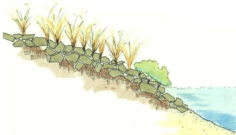
Figure 9 - Improvement Example, Vegetate Existing Stabilization Feature
